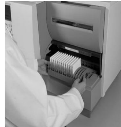
Figure 4. VITEK 2 Cassette Loaded with Cards and Suspension Tubes Being Loaded Into the Automatic Transport System.
